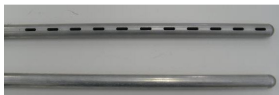
Fig. 2 Cylinders with and without periodic holes
